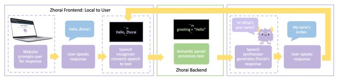
Figure 2: A representation of the introduction to Zhorai in terms of architecture and user flow.
