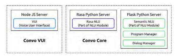
Figure 4-1: A diagram showing the servers and components that make up Convo. In total, there are three servers and four main components.
