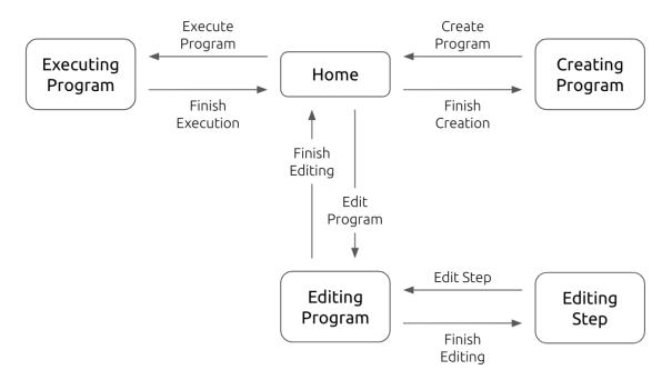
Figure 4-4: The diagram depicts the state machine in the dialog manager and the transitions between the states. Users first start in the Home state and transition to the other shown states with different intents.
