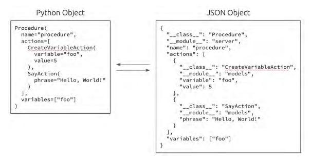
Figure 4-8: An example procedure with its Python object representation and JSON object representation. The additional metadata fields in the JSON object are necessary for the conversion back to a Python object.
