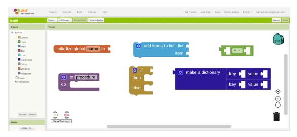
Figure 4.2.: MIT App Inventor blocks editor for adding logic and behavior to App components
