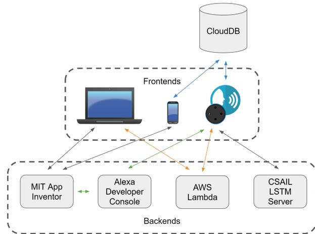
Figure 6: The architecture for the conversational AI interface. This is discussed in more detail in (Van Brummelen 2019).
