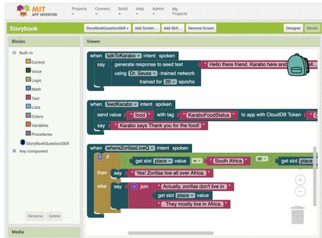
Figure 4: Sheila’s storybook endpoint function blocks in MIT App Inventor. Notice the *when intent spoken*, *say*, and *generate text* blocks.
