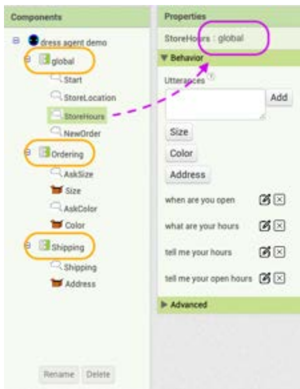
Figure 6-2: Mockup for the improved Components panel (left) and Properties panel (right) in the Designer editor.
