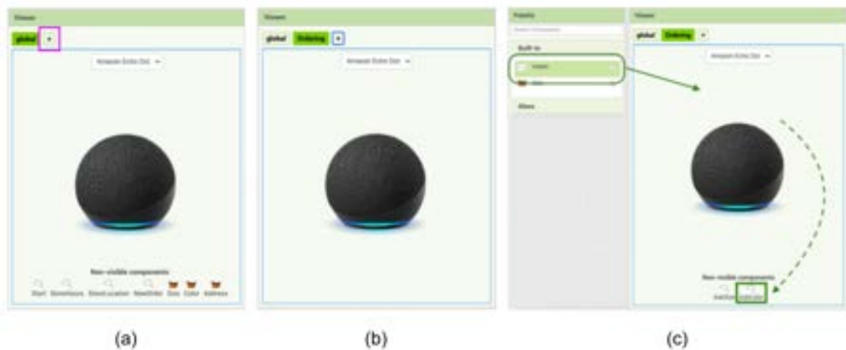
Figure 3-7: (a) Viewer panel in the Designer page before intents are added for the 'Ordering' state. (b) Viewer panel after intents are added for the 'Ordering' state.
