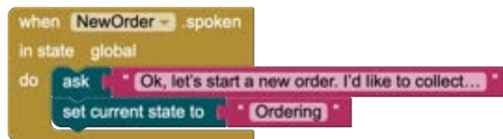
Figure 3-12: The endpoint event for the NewOrder intent. These blocks cause Alexa to respond with the sentences attached to the Ask block and change the current state of the conversation from 'global' to 'Ordering' .
