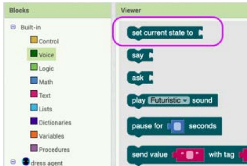
Figure 3-11: The “Voice” blocks drawer for all Alexa-related blocks. The purple box highlights the set-current-state block.
